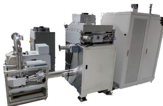
A single cavity equipment with the atomic layer deposition (ALD) and atomic layer etching (ALE) double processes
