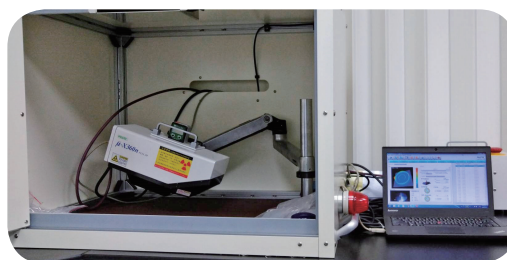
Residual stress on curved steel surface
