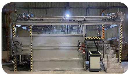
CV flow test equipment
