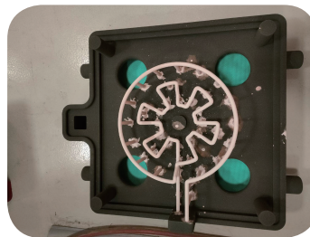
Sand mold with high slenderness ratio of the inner runner
